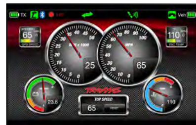
The customizable Traxxas Link dashboard delivers real-time rpm, speed, temperature, and voltage data.
